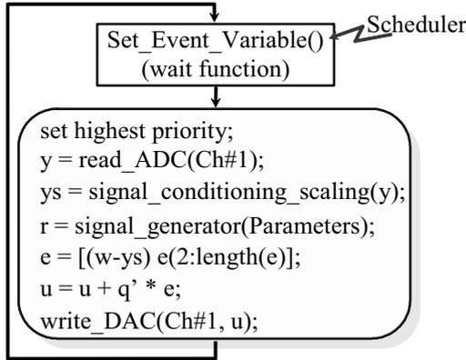
Figure 4. Controller implemented with one real-time periodic task
