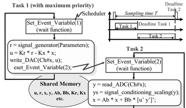
Figure 6. Real-time implementation of a state-space controller
