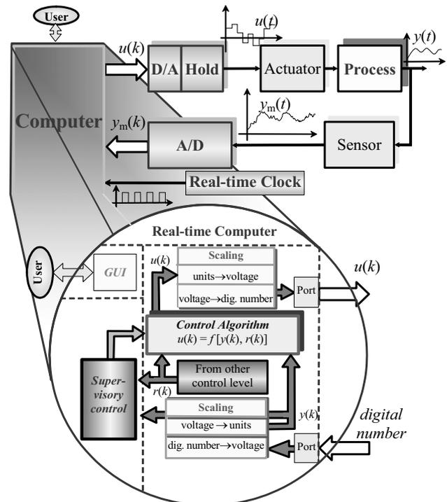
Figure 1. Overview of a computer controlled system
