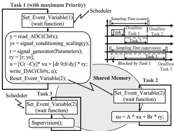
Figure 7. Real-time implementation of a state-space controller
