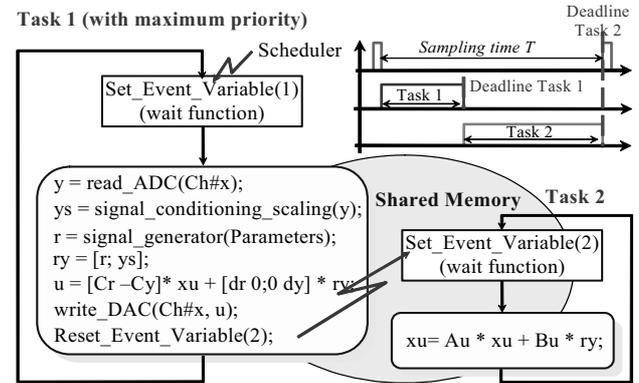
Figure 5. I/O Controller implemented with two real-time tasks
